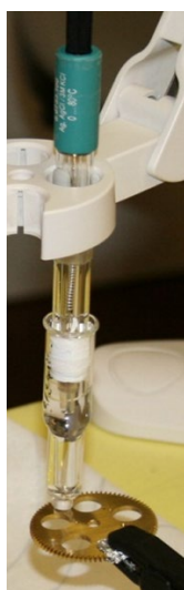
Fig. 2: The measuring system RE / junction tube.
