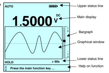
The graphical window and the bargraph constantly track the evolution of the measurement in the range selected.
