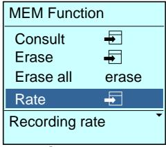
• Validation of Rate with the weep key opens a menu for setting the required recording rate in hours, minutes and seconds:
