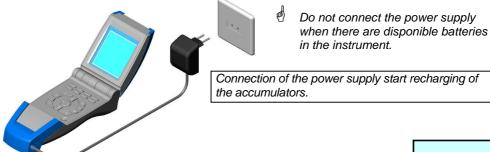
Connection of the power supply start recharging of the accumulators. The symbol shows the progress of recharging.
