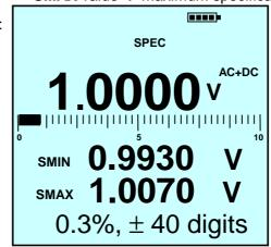
In AC+DC, the specifications are calculated only if the frequency can be measured (see §. secondary Functions) and is > 45 Hz.
