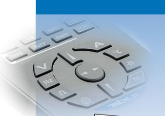
For even more detail, the **MEM key** records up to 6,500 time/date-stamped measurements at intervals ranging from 1 s to 24 h so that they can be analysed graphically on the instrument. This function can be used for 1, 2, 3 or even 4 simultaneous measurements.
