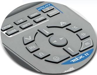
A "favourite measurement" key allows users to program automatic access to the measurement mode they use the most. Whatever the physical quantity measured, this key enables you to convert the scale and define the appropriate measurement unit in order to obtain direct readings of the original quantity.
